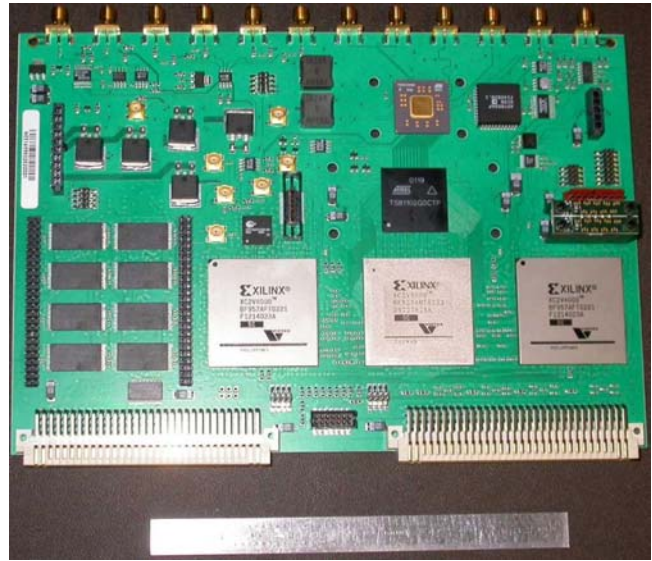
Figure 1 LNX 's Digital Receiver module can sample at rates up to 2 Gsa/sec and accommodates up to three Virtex-II FPGAs for real-time DSP applications.
